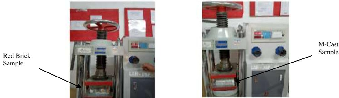
Figure 3. Compressive Strength Testing
